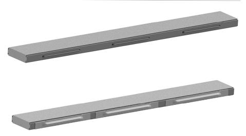
9 Slide the mesh pack back into the pullbar. Make sure the cords that go through hole 1,2,3 come out at side B and cords that go through hole 4,5,6 come out at side A
