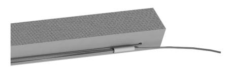
Place the cord tensioner on the end of the cord and secure it with a knot. Do this for both sides.
