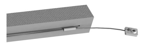
Place tape on the back of the mesh pack to insure the cord stays in position.
