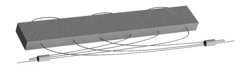
Pull on the cords so they are all tight when the cord connector is placed against the mesh pack at the last hole on both sides.
