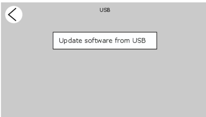
Once the firmware is ready to be installed, the button changes color to white. Now tap the button and the display will show bootloading. This will take approximately 30-60 seconds\*, depending on the size of the update.
