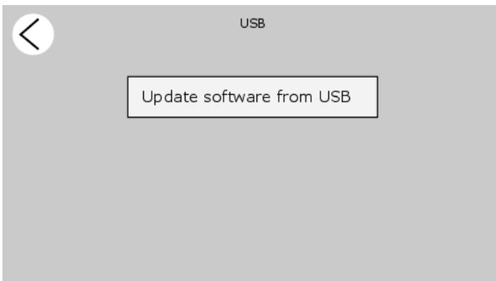
During the loading of the firmware the button 'Update software from USB' is grey.
