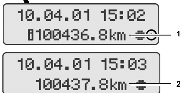
Fig. 5-19: MTCO 1390: Odometer reading, example of odometer check
