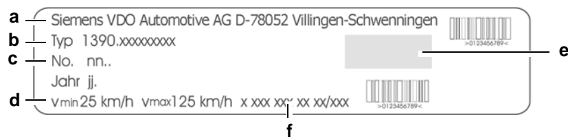
Fig. 2-4: MTCO 1390: Type plate (general)
