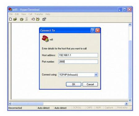
(4) Once connected with a proper IP address, you should get the response \*HELLO\*. Input escape sequence \$\$\$ to make the WiFi module enter commands mode, and Hyper Terminal should returns CMD to you.
