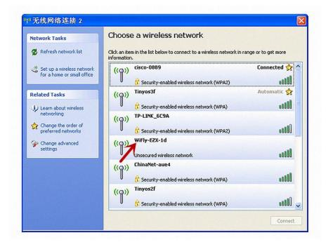
**NOTE:** It may take a while for Windows to connect to the network and assign an IP address. You can check the IP address of your computer by running the ipconfig command in the command window. Once connected, this command will show you the IP address and net mask.
