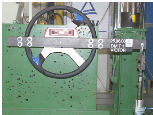
Torsion test (see section 3.1.5.); Steering wheel 3L450 "A" (representative test)
