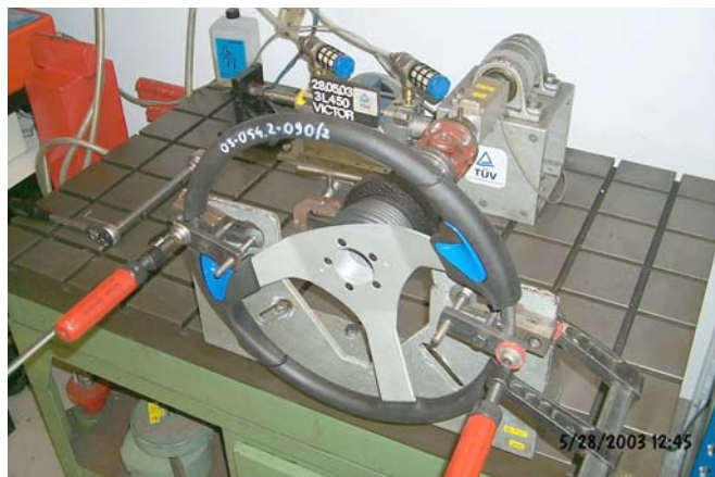
Fatigue test (see section 3.1.4.); Steering wheels 3/4L450 "A" (representative tests)
