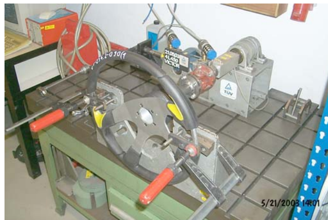
Fatigue test (see section 3.1.4.); Steering wheels 3/4L450 "A" (representative tests)
