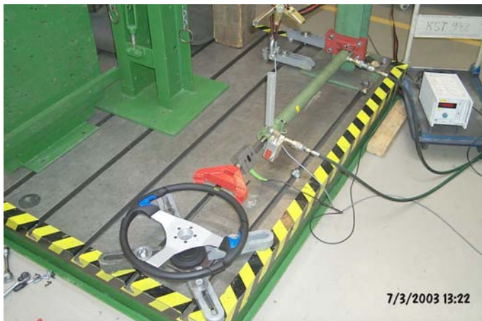
Static deformation test (see section 3.1.1.); Test facility
