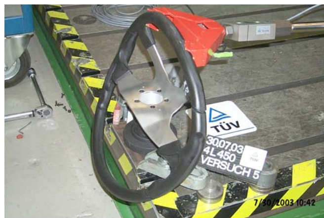
Static deformation test; Steering wheel 4L450 "A" (representative test)
