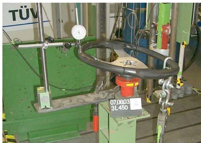
Bending test (see section 3.1.2.); Steering wheel 3L450 "A" (representative test)
