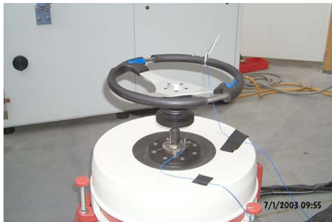
Vibration test (see section 3.1.3.); Steering wheel 3L450 "A" (representative test)
