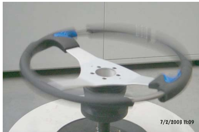
Vibration test (see section 3.1.3.); Steering wheel 3L450 "A" (representative test)
