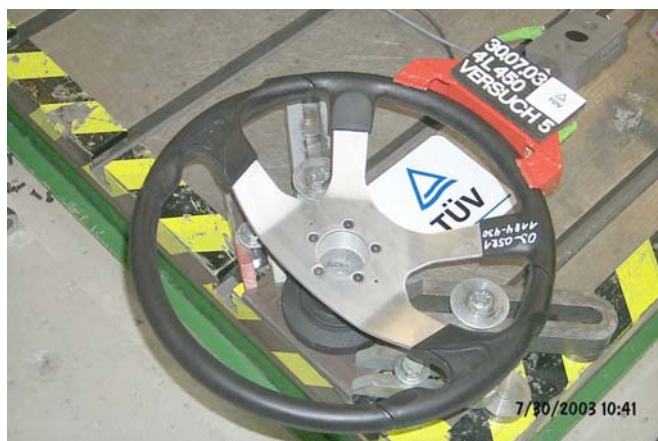
Static deformation test; Steering wheel 4L450 "A" (representative test)
