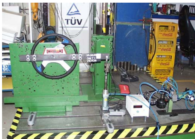
Torsion test (see section 3.1.5.); Steering wheel 3L450 "A" (representative test)
